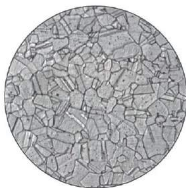
3系不銹鋼金相 Microstructure for 300 Series.
