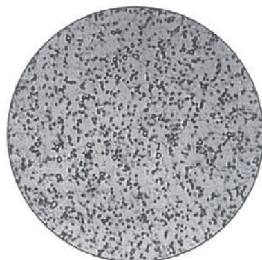
SCM435金相 Microstructure for SCM435
